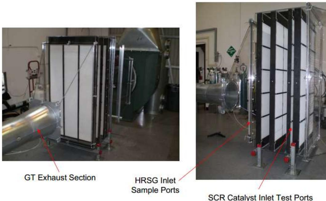
Figure 5. 1/16 Cold Flow Model (courtesy of FERCo)
