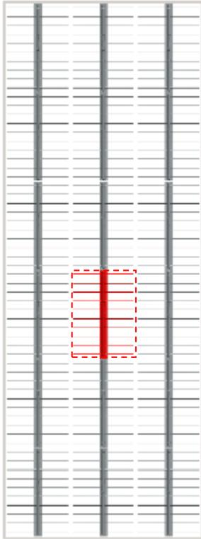
Figure 3: Three-Zone AIG Arrangement Elevation (Left) and Conceptual 3D Model (Right) (Horizontal HRSG)
