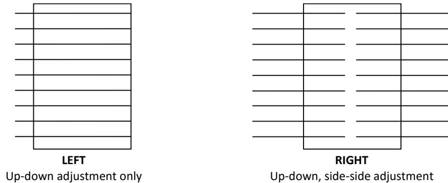
Figure 2: One- & Two-Zone AIG Arrangement Sketches
