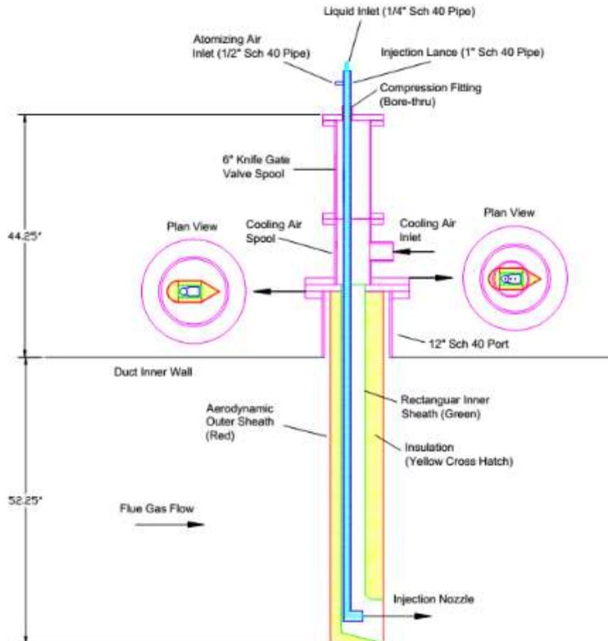
Figure 6. Schematic Showing Implemented Lance & Sheath Design for Jingfeng
