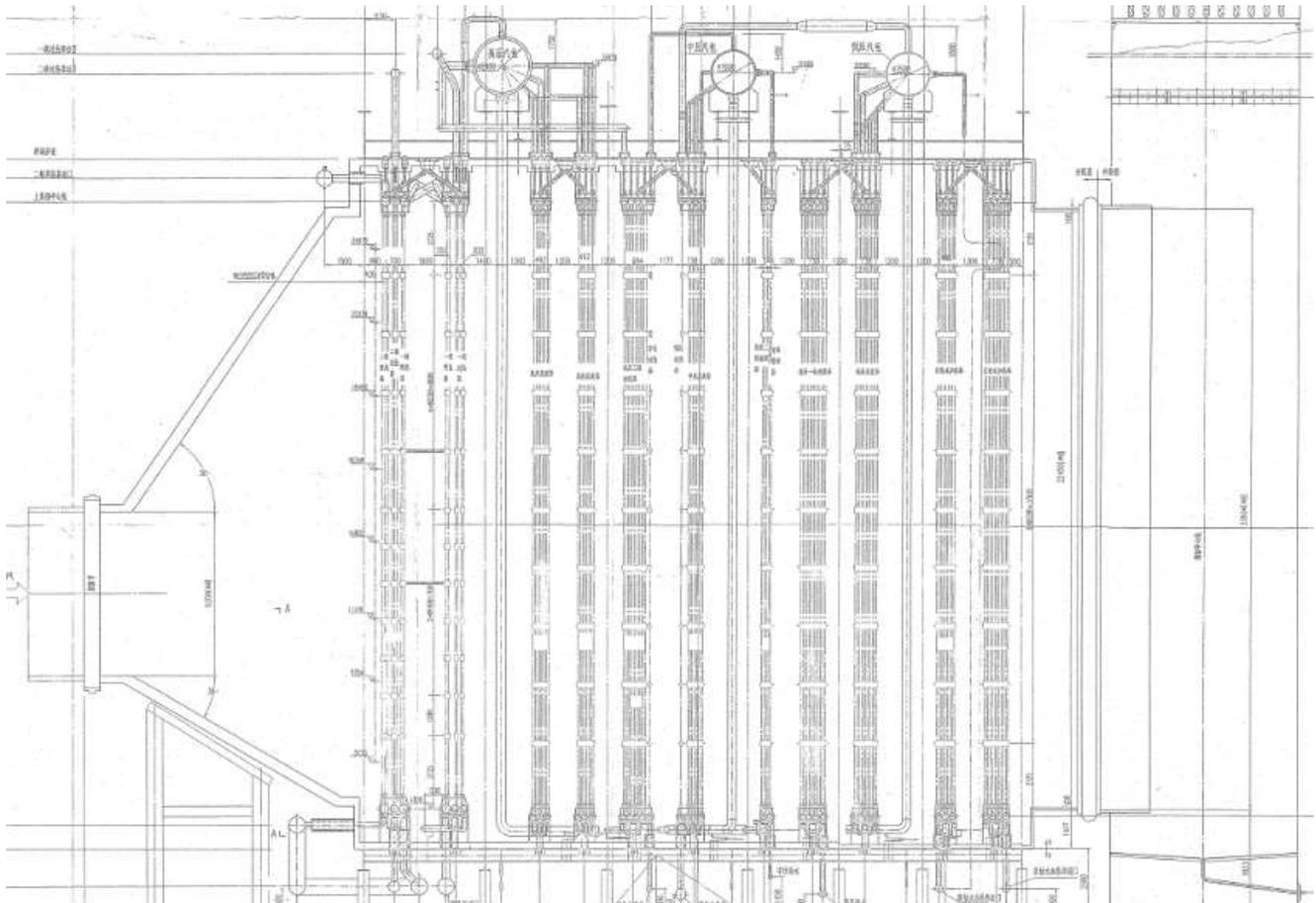
Figure 4. Elevation Drawing of HRSG Showing Lack of Emissions Casing Section [courtesy of Jingfeng Power Plant]
