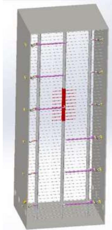
Typically, the OEM will leave 8 to 10 feet from the AIG to the face of the catalyst to allow for proper mixing. The end result is a costly grid of piping and large empty cavity in the HRSG. One US OEM has estimated that removing the AIG and SCR cavity would allow them to remove a column line and reduce casing around the “emissions cavity” by roughly 50% [3], leading to significant capital cost savings during the construction of a new combined-cycle power plant.
