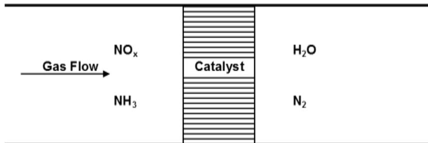
Figure 1. Schematic of SCR Process
